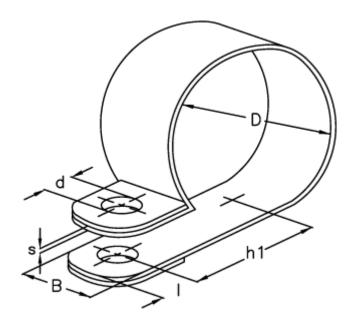
$\begin{array}{ll} d & = 8.4 \\ \text{Diameter D} = 9 \\ \text{h1} & = 17.0 \\ \text{I} & = 8.5 \\ \text{s} & = 0.8 \\ \text{Width B} & = 20 \\ \end{array}$
